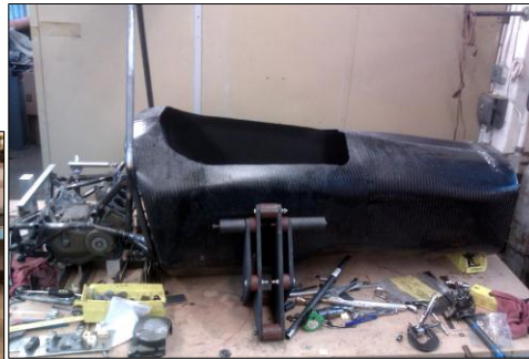
Above: Team 22 half monocoque, half spaceframe chassis during assembly
